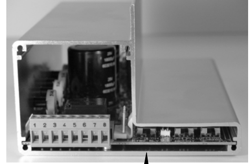
LATCH DELAY OFF/ON SWITCH
